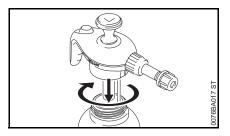
Fit the cover and tighten it down firmly.
