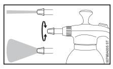
Rotate the nozzle to adjust the spray pattern (solid jet or fine mist).
