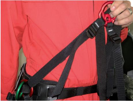
Pass the webbing of the two Legs of the Lower Part under the top of each of the two Lying Rings on the treeMOTION
