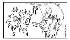
Rotate the inner right-hand blade (4) on the shaft until it can be pushed into position – check the direction of rotation again (arrows).
