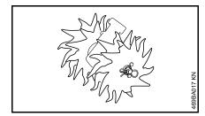
Pick tines are particularly suitable for tilling and loosening hard or packed soil.
