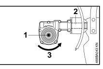
Gearbox output shaft (1) below the drive tube (2).
