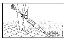
Always hold the power tool firmly with both hands on the handles. Right hand on control handle, left hand on loop handle on drive tube, even if you are lefthanded. Wrap fingers and thumbs firmly around the handles.
