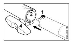
Push the lug (1) on the drive tube into the slot (2) in the coupling sleeve as far as stop.
