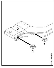
Insert square nuts (1) in the barrier bar (2) – the holes must line up
