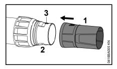
Push the nozzle (1) onto the blower tube (2) and engage it on the lugs (3).
