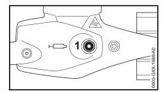
Check the lubricant level at regular intervals of about every 25 hours of operation. Unscrew the filler plug (1) – if no grease can be seen on the inside of the filler plug, screw the tube of grease into the filler hole.
