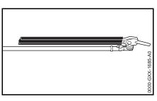
The cutter bar can be folded flat against the drive tube and locked in position to save space during transportation.
