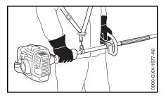
Right hand on control handle, left hand on loop handle on drive tube, even if you are left-handed. Wrap fingers and thumbs firmly around the handles.
