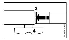
When correctly installed, the red line (3) (arrow point) must be flush with the end of the coupling sleeve.
