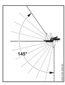
The angle of th cutter bar can be adjusted upwards in 4 stages from  $0^{\circ}$ (straight) to 55°, and downwards in 7 stages from 0° to 90° (right angle facing down). There are therefore 12 possible working positions.
