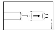
Pull the protective cap off the end of the drive tube and keep it in a safe place.
