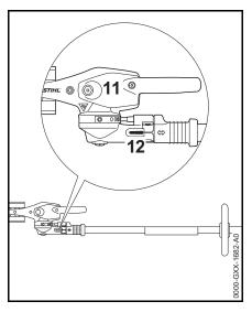
Once the end of the drive tube is inserted beyond the slot in the clamp (12):
