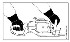
Left hand on the control handle and right hand on the front handle.
