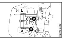
• Adjust idle speed with the idle speed screw (LA) so that the cutting blades do not run.
