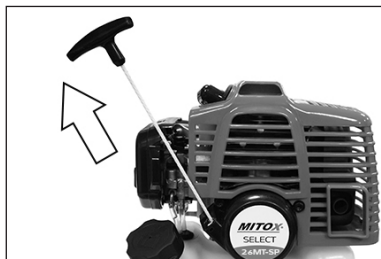
Fig 6 - Pull the starter rope until the engine starts, then squeeze the throttle briefly to release the fast idle control and return the engine to idle.
