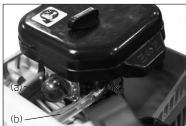
Fig 1 - Push the air purge bulb (a) until fuel is visible in the clear return fuel line (b)
