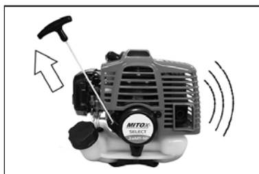
Fig 4 - While holding the unit, pull out the starter rope firmly until the engine fires (indicated by a 'cough' from the engine).
